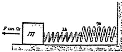
**Problem #2.** Determine the natural frequency of each of the systems shown. Are there any values of the spring stiffness  $k$  for which either system will not oscillate freely about the vertical position?
