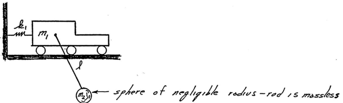
Problem #2 Determine the equation of motion for the system shown. Find an expression for the critical damping coefficient.
